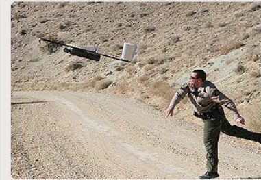
Mesa County, Colo.'s fixed-wing drone can be launched by hand and fly for up to an hour. Click here to read more about how drones can assist in search and rescue missions.
